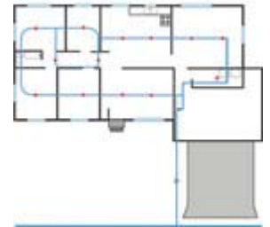
Simple looped multipurpose system installation. Piping must be installed with no dead ends to ensure a non-stagnant system.
